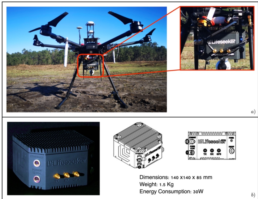
Figure 1: a) Example of IMSI Catcher technology equipped on UA DJI M600 of CNVVF. b) IMSI Catcher system and main characteristics.
