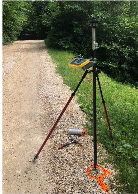
Fig.2.2.3.2 Prism 360 - con controller TCU 3-
