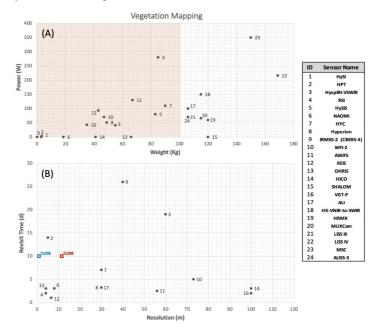
**Fig. 1.** (A) Scatter-plot of weight and power values of the satellite sensors supporting vegetation mapping applications. The red area encloses values fulfilling CLOSE mission requirements. (B) Scatter-plot of spatial resolution and revisit time of sensors lying within the red area in plot A. Number labels correspond to sensors according to the table on the right side.
