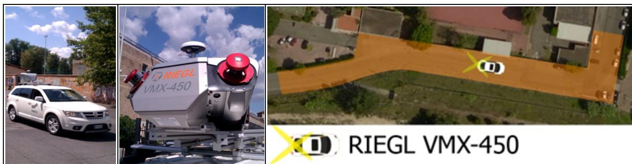
Figura 4 - Laser Scanner Mobile Riegl VMX-450
